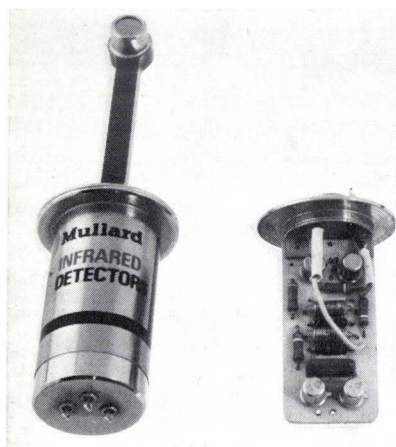
Fig. 14. Various types of pyroelectric infrared detector made by Mullard Southampton. All these detectors contain crystals of alanine-doped TGS. Top picture: the most usual configuration (see fig. 13). Left: a version in which the crystal is mounted on the end of a short post, for a special application. Immediately above: an experimental miniature detector in a TO5 package, consisting of 128 detectors on one crystal, each detector with its own amplifier; the connector strips can be seen in front of the housing and behind it.
