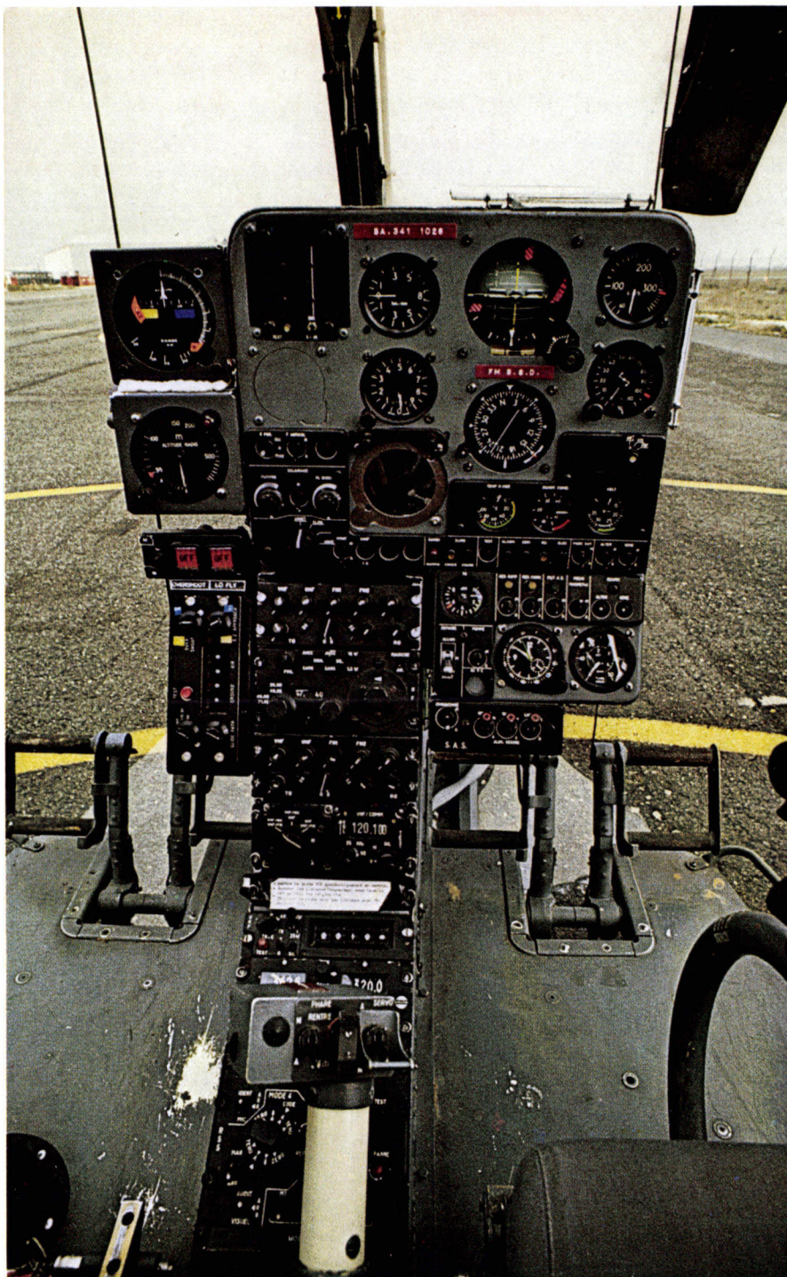
Fig. 6. Instrumentation in a MADGE-equipped Gazelle helicopter. Top row, second from right: two-axis horizon; the crossed pointers are actuated by the MADGE azimuth and elevation guidance outputs. Top row, at left: display developed for MADGE; a radial pointer indicates range up to 30 n miles on a nonlinear scale; an edgewise pointer gives azimuth deviations from the MADGE centre-line up to \pm 45^\circ . Bottom left: pilot's controller (see 4 in fig. 5). Above this: 'doll's-eye' indicators for safe elevation angle and overshoot sector indication.
