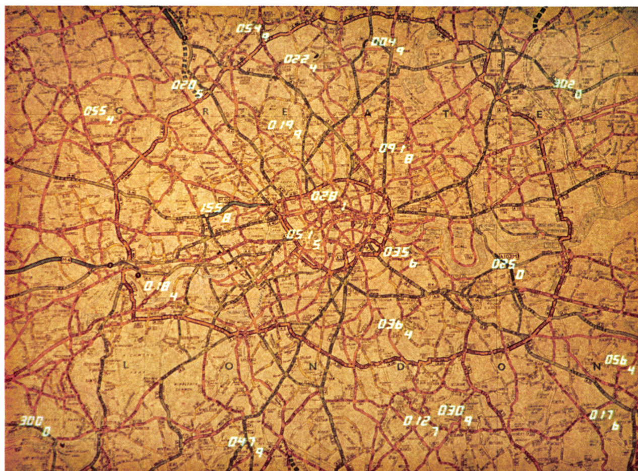
Fig. 7. Photograph of location display on a map of central London. The three-digit numbers are the vehicle identification numbers and the suffix is a status number (e.g. busy, free, returning to base, etc.). The actual location of each vehicle is marked by the suffix digit.
