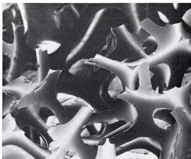
Fig. 20. Demonstration of the effect of the aperture angle of the scanning electron beam on the depth of field. As in fig. 1 , the object is a plastic foam coated with a gold film. The three pictures were made with a distance of 23 mm between the diaphragm of the objective and the specimen. The aperture diameters were, downwards, 400 \mu\text{m} , 200 \mu\text{m} and 100 \mu\text{m} . An aperture of 100 \mu\text{m} was also used in making the photograph for fig. 1 , but the distance between diaphragm and specimen was 43.5 mm. The depth of field was also correspondingly greater. Magnification 75 \times .
