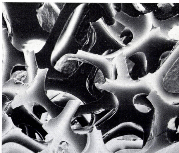
Fig. 1. Scanning-microscope picture of plastic foam, coated with an extremely thin gold film for this picture. The depth of field is clearly much greater than the resolving power. This is different from optical microscopy, where the two quantities are approximately equal. Magnification 75\times .
