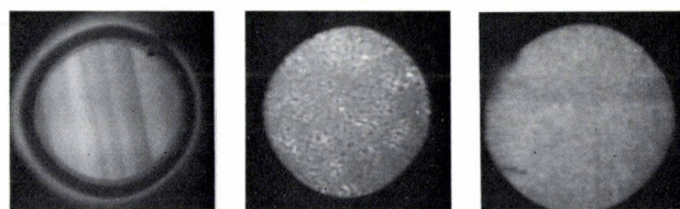
Fig. 8. Photocurrent distribution for diodes made from silicon of different quality. The right-hand picture shows the current distribution of a diode whose P - N junction was made by ion implantation in epitaxial silicon.
