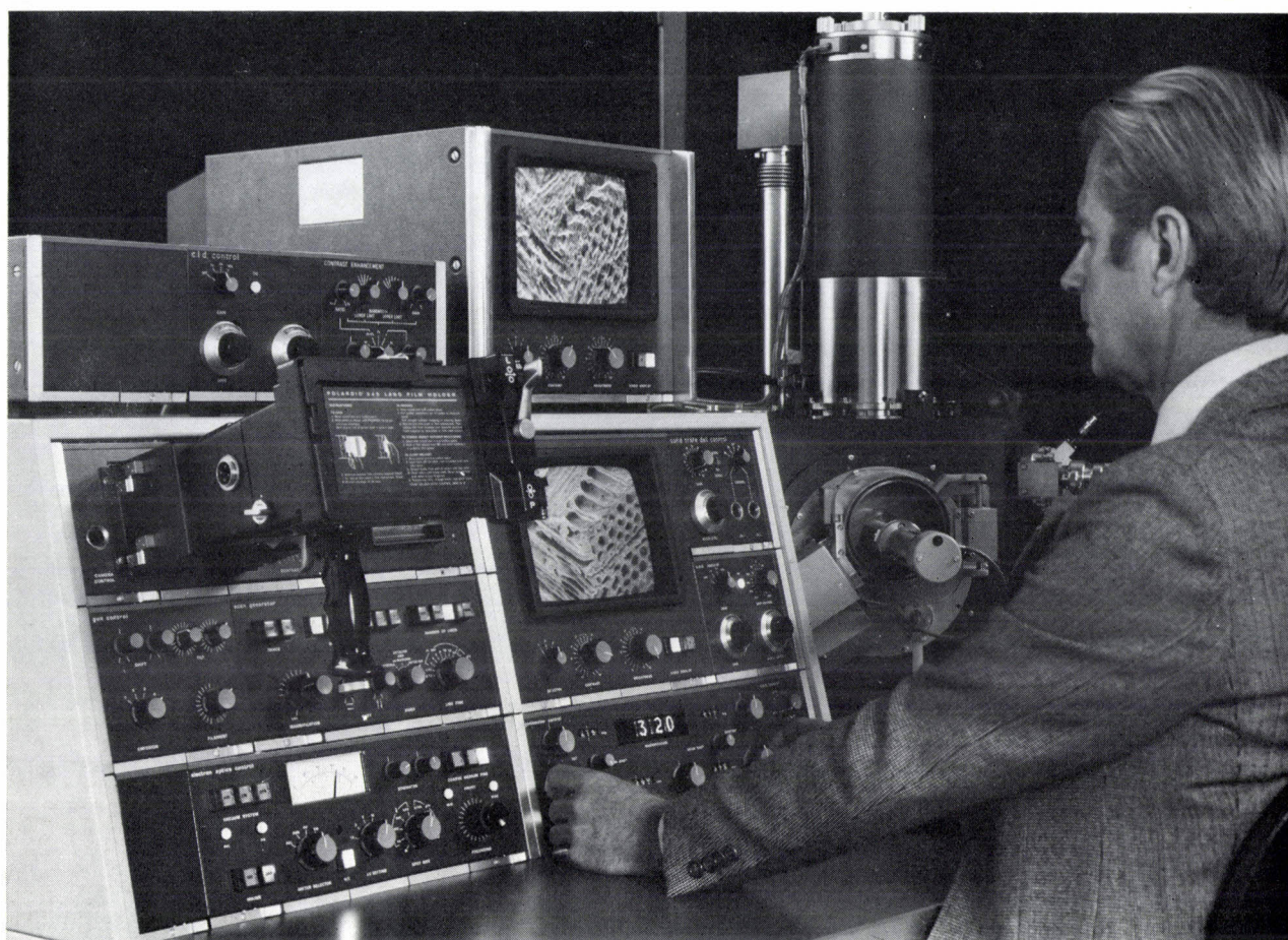
Fig. 9. The control panel of the PSEM 500. The standard range of control units has been extended by the addition of a number of optional units. The units at the extreme right of the panel are (from top to bottom) the control units for solid-state detectors (as used for the detection of back-scattered electrons), for the secondary-electron detector, which is part of the standard equipment, and for the detector for absorbed electrons (specimen current). A control unit for a cathodoluminescence detector and the circuit for electronic contrast enhancement are included as separate units on top of the panel, at the left. Finally, an extra cathode-ray tube has been included, used here to display a picture with 'y modulation'. In this kind of presentation the detector signal gives a vertical deflection of the electron beam producing the picture, rather than an intensity modulation.
